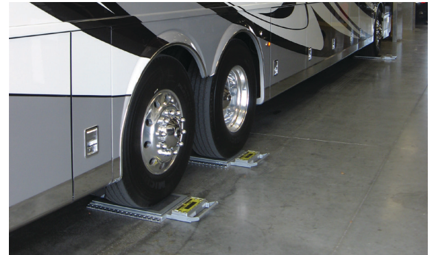
Individual wheel weights, axle weights and GVW (Gross Vehicle Weight) can be determined using an LP600™ scale pad under each wheel.
